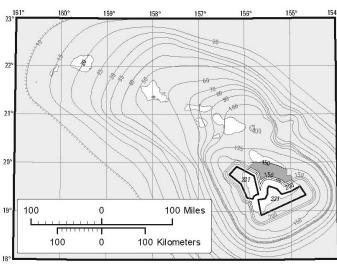
0.2 Second Spectral Response Acceleration (5% of Critical Damping)
