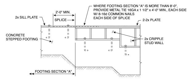
NOTE: WHERE FOOTING SECTION "A" IS LESS THAN 8'-0" LONG IN A 25'-0" TOTAL LENGTH WALL, PROVIDE BRACING AT CRIPPLE STUD WALL
