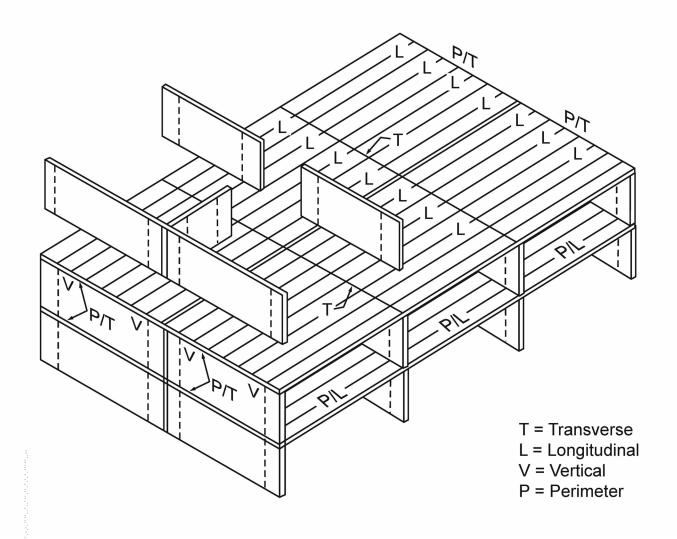
FIGURE 1615.4 LONGITUDINAL, PERIMETER, TRANSVERSE AND VERTICAL TIES
