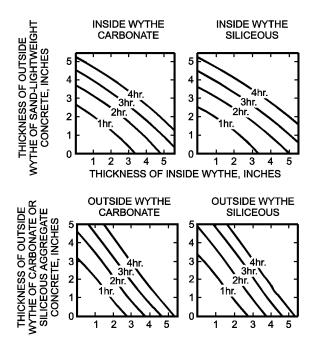
THICKNESS OF INSIDE WYTHE OF SAND-LIGHTWEIGHT CONCRETE, INCHES
